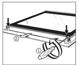
Unscrew the Torx screws and then pull the guides and the trim together with the seal off.
